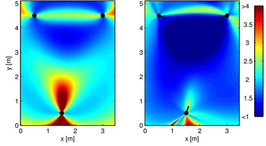
Fig. 3. Root CRLB, see eq. (14), in [m]: Comparison between model with omnidirectional characteristic (see eq. (1)), left figure; and angular dependent model with parameters from lab measurements (see eq. (2)), right figure.
