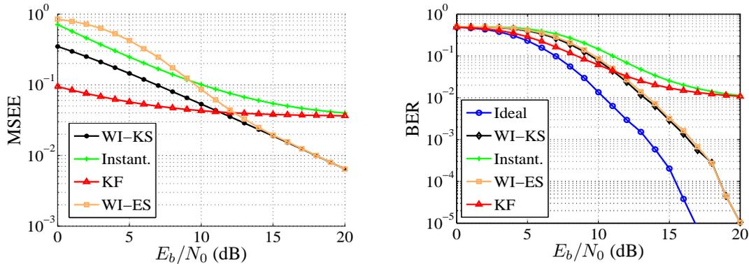
**Fig. 1.** Wiener interpolation in time direction by assistance of a pre- and generated postamble: channel model with six propagation paths of  $[-6.5, -7.6, -8.7, -9.8, -10.9, -12.0]$  dB and delays of  $[0, 50, 100, 150, 200, 250]$  ns.
