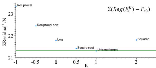
Fig. 10. Statistical Box-Cox-plot for shear force indicating that untransformed shear force measurements have the most accurate model. Green line illustrates 95% confidence interval of residual squared.
