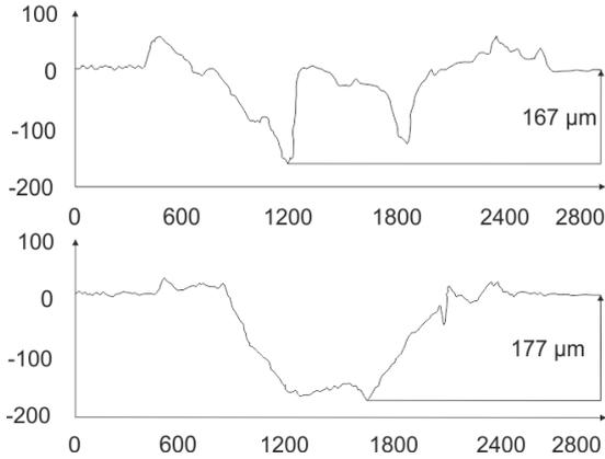
Fig. 8. Residing imprint of pin with cracks from shearing (top) and residing imprint of rotated pin (bottom)
