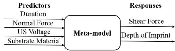
Fig. 6. Meta-model illustration showing meta-model with predictors and responses
