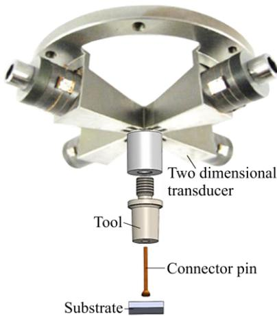
Fig. 2. Detailed view of the two-dimensional bonding system
