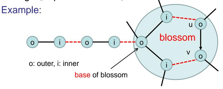
If for some outer (resp., inner) node u an edge {u,v} is found where v is already an outer (resp., inner) node, then we have an odd cycle, called a blossom.
