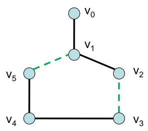
Definition 5.6: An alternating path w.r.t. a matching M is called augmenting if it contains unmatched nodes at both ends and does not form a cycle.
