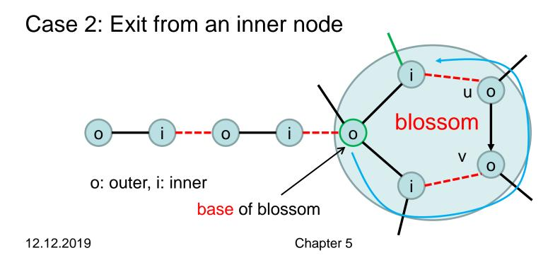
Invariant: for each contracted node, there is an internal alternating path from its base to any of its edges, starting with a non-matched and ending with a matched edge.
