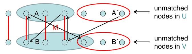
Define A⊆U: nodes reachable via alternating paths starting in A´ Define B⊆V: nodes reachable via alternating paths starting in A´ Observations:
