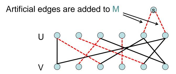
Note: Adding s has effect of running DFS from all unmatched nodes in U in parallel – hence O(m+n) time per augmenting path found
