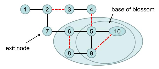
Solution: recursively find an augmenting path from base of blossom to the exit node.
