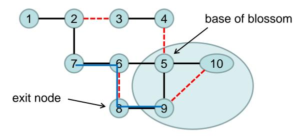
Solution: recursively find an augmenting path from base of blossom to the exit node.
