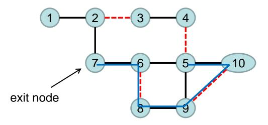
Solution: recursively find an augmenting path from base of blossom to the exit node.
