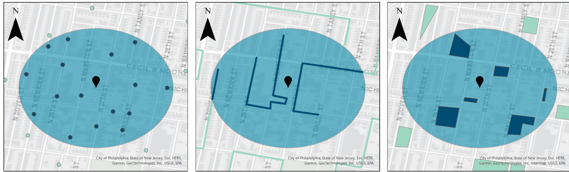
Figure 4: GIS buffer analysis for point (left), line (middle), and polygon (right) objects.
